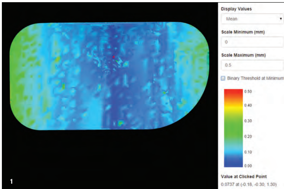
Figure 1: Heat map comparing the Victory Series™ Superior Fit Buccal Tube 1st Molar Base with representative tooth surface.
