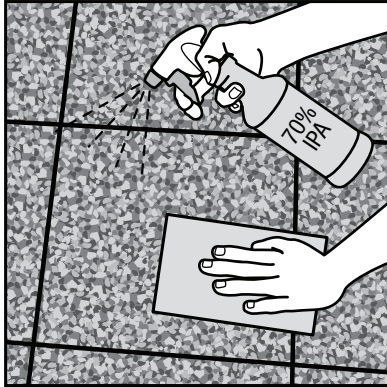
Figure 1 Clean surface by using a dampened paper towel with 70% Isopropyl Alcohol Solution (IPA).
