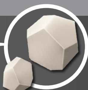
As the resin wears, large and unevenly sized filler particles are exposed. This creates a rough and uneven surface as they break away from the resin matrix.
