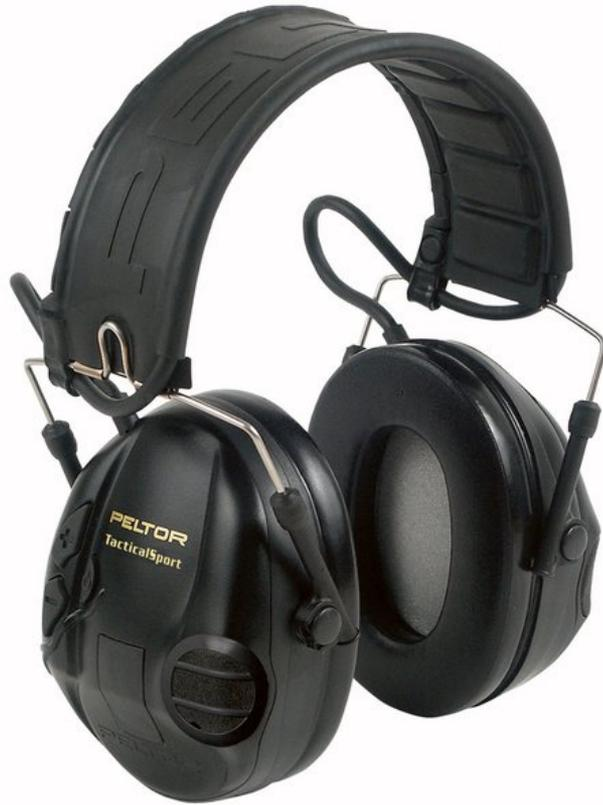
The Tactical Sport Hearing Protector electronic earmuff uses proprietary integrated circuit technology for a refined audio reproduction. It gives users fast shutoff and recovery time while helping protect hearing from harmful impulse noises, such as gunfire. Sound amplification allows the user to hear low-level sounds, including range commands and conversation.
