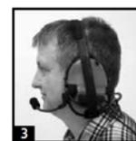
**3:** Take the velcro straps attached to each headset and bring over the head and fasten together, ensuring each ear cushion remains over the ear and is supported by the head strap.
