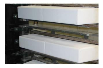
Furnace door casing to prevent the erosion of bulk fibre insulation material.
