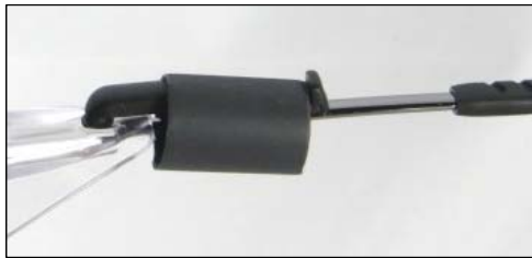
3M™ heat shrink tubing slipped over locking bar and temple
