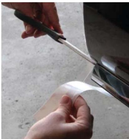
7. Begin pressing the film around the edge of the door over the entire length of the door, but not all the way to the back side yet. This will help to prevent air bubbles.
