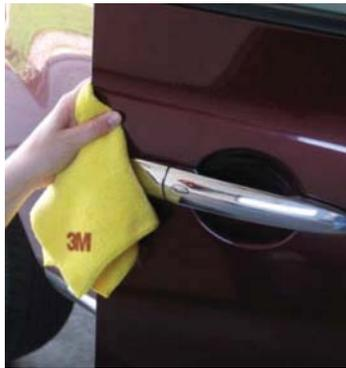
3. Always check part position, shape and size before applying. The Door Edge film is rounded on the ends; if desired it can be cut straight.
