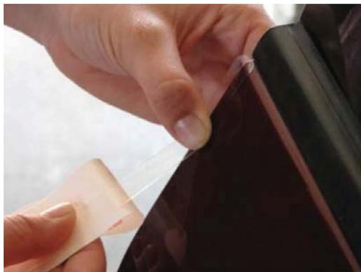
6. Continue this process down the door edge to the bottom of the film. Trim at the bottom as necessary with scissors or razor blade.
