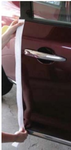
4. Start to remove one strip from the paper. Do not pull the entire strip off the paper as the adhesive can become contaminated.
