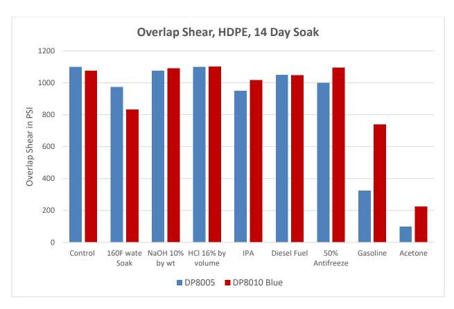
Bonding Strength of 3M<sup>TM</sup> Scotch-Weld<sup>TM</sup> Structural Plastic Adhesive DP8005 and 3M<sup>TM</sup> Scotch-Weld<sup>TM</sup> Structural Plastic Adhesive DP8010 Blue on HDPE after various environmental challenge conditions.
