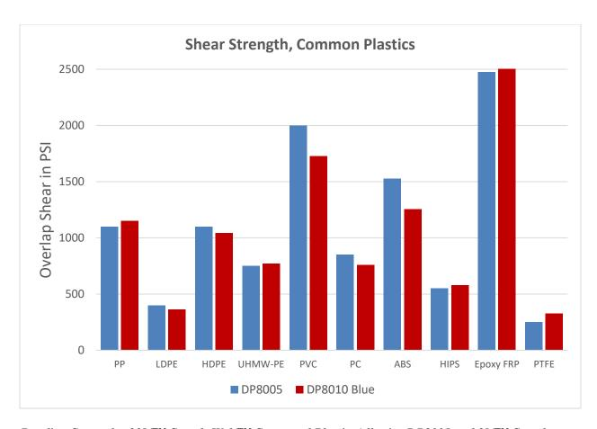
Bonding Strength of  $3M^{\rm TM}$  Scotch-Weld<sup>TM</sup> Structural Plastic Adhesive DP8005 and  $3M^{\rm TM}$  Scotch-Weld<sup>TM</sup> Structural Plastic Adhesive DP8010 Blue on some common plastics.
