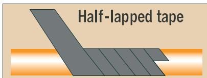
Half-lap tape application enhances adhesion and insulation functionality.
