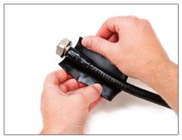
4.3 Starting 1" (25 mm) below the butyl mastic tape, wrap one half-lapped layer of 2" (51 mm) vinyl tape up to the connector clamping nut. Repeat procedure to apply second half-lapped layer.
