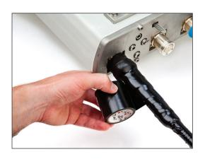
3.5 Starting 1" (25 mm) below the previous layer of vinyl tape, wrap the entire cable and connection section with three continuous half-lapped layers of ¾" (19 mm) wide vinyl tape.
