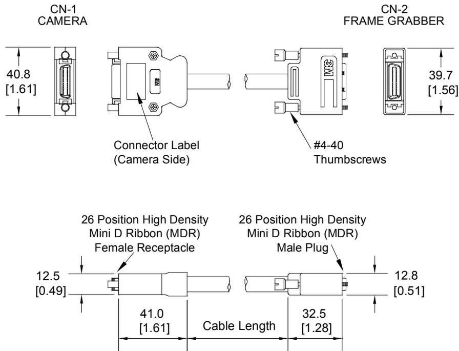
Cable Length Tolerance is the Larger of +50mm / -0mm or +3% / -0%
