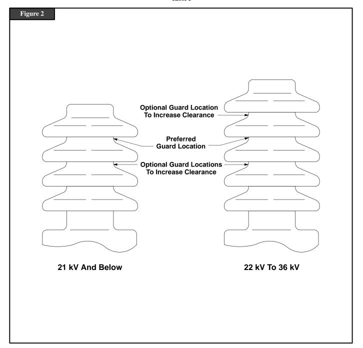
NOTE: Under no circumstances should a guard be forced onto an insulator.
