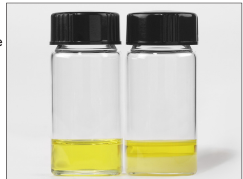
Figure 3. (l) Nanofiller in 3M™ Adper™ Single Bond Plus Adhesive remains in solution; (r) filler in Optibond Solo Plus™ does not.
