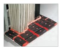
12.5 3M™ Fire Protection Self-Locking Pillows are completely reusable. Simply remove the desired pillow(s) by inserting fingers on both sides. Squeeze gently to release the interlocking bond and remove the pillow. For wall configurations no additional support required (e.g. wire mesh or steel cover plates).
