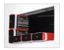
12.2 Combine self-locking pillows at interlocking strips. Compress pillows to 33%. Insert and install in groups into the wall.
