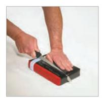
13.2 Resealing 3M™ Fire Barrier Self-Locking Pillows can be accomplished by using either the removed original outer cover, minus contents, or by use of two inch wide carton sealing/packaging tape.
