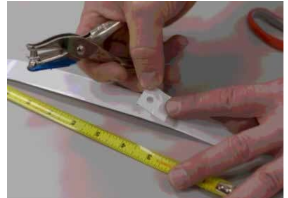
Figure 2. Preparing the test strips
