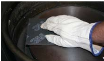
1. Thoroughly clean and dry the platen. Scotch-Brite™ Pads work well to remove debris and oxidation.
