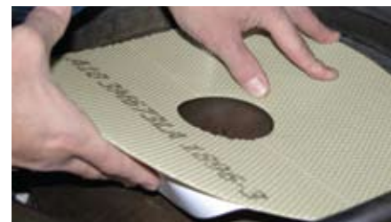
2. Position the abrasive, hold in place, remove one edge of the liner, and fold it under the abrasive.
