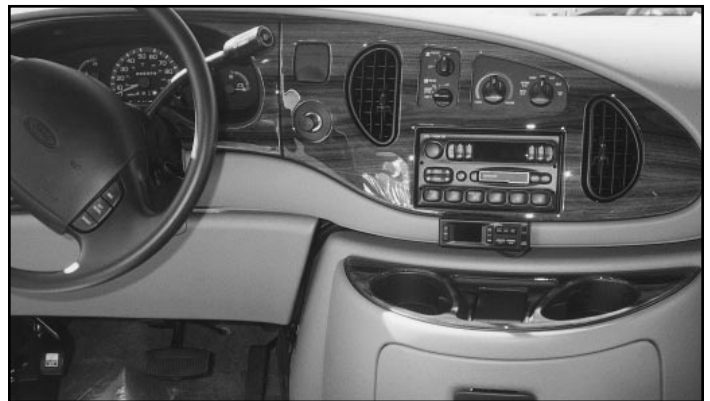
Interior wood dashboard kit from Accu Laser Technologies installed in a 1997 Ford Econoline Club Wagon XLT. When attached with 3M™ Acrylic Foam Tape to properly cleaned and primed dash surfaces, wood trim lends a look of class that lasts the vehicle’s lifetime.
