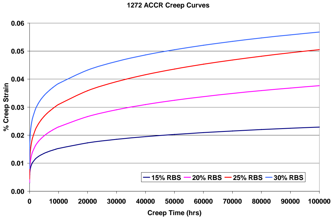
Figure 5. Creep strain vs. time for 1272-kcmil conductor at all test loads
