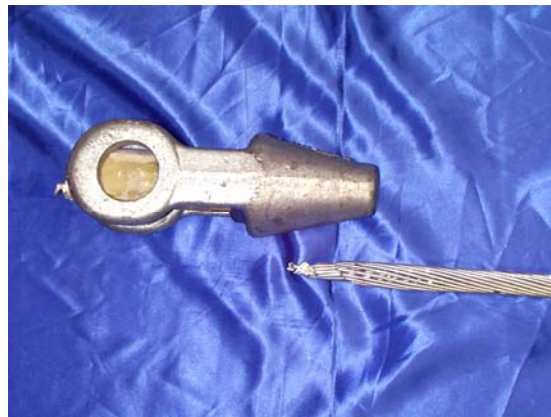
A typical conductor failure at the epoxy end
