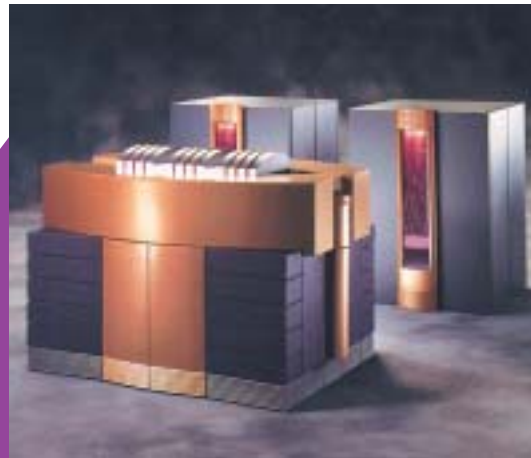
Direct contact cooling with 3M™ Fluorinert™ Electronic Liquids helped enable the development of dense electronics, such as supercomputers.
