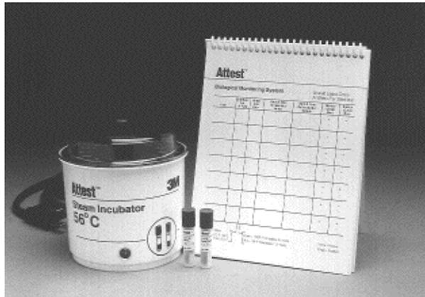
1261P Attest™ biological indicators were designed to monitor 270°F/132°C gravity “flash” steam sterilization processes. Special spore strip placement and cap design on the 1261P Attest™ biological indicator provide a more representative challenge to the 270°F/132°C gravity displacement steam sterilization cycle.
