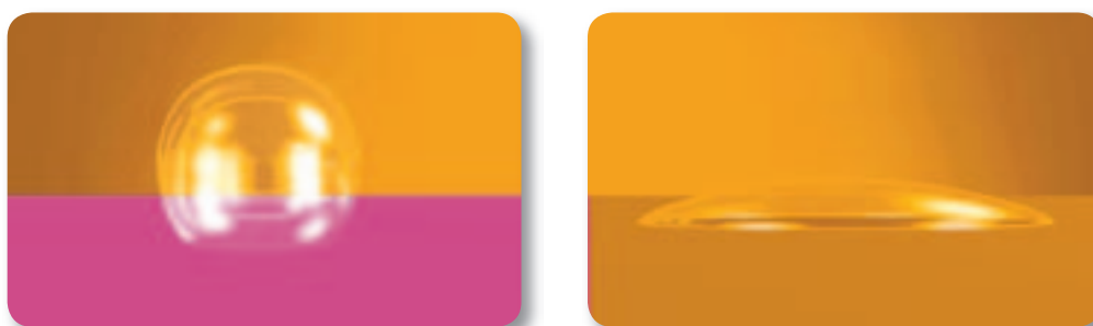
Fig. 5: Hydrophobic (left) versus hydrophilic behaviour of a water droplet on impression material (schematic pictures).
