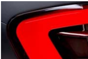
Caption: A closeup of the lighted cavity shows the consistency of light as it wraps around a tight corner, enabling design flexibility of tail lamps.
