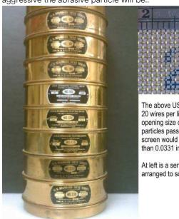
The above US standard screen has 20 wires per linear inch giving an opening size of 0.0331 inches. All particles passing through this screen would have a size of less than 0.0331 inch.
