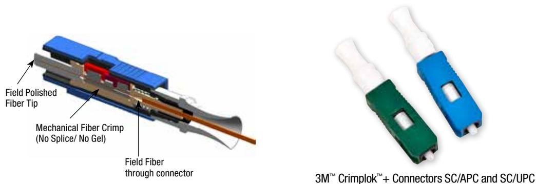
The connectors are SC-compatible and contain a metallic element which mechanically locks the fiber in place. Crimplok+ connectors have a thermally-balanced design that has been tested for premises and FTTP applications and for indoor and outdoor conditions ranging from -40° F to 167° F (-40° C to 75° C).
