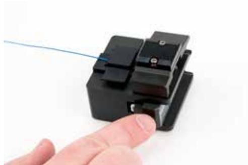
**Step 2 – Insert cleaved fiber through Crimplok+ connector and lock into place, using the 3M™ Crimplok™ + Protrusion Setting Tool**
