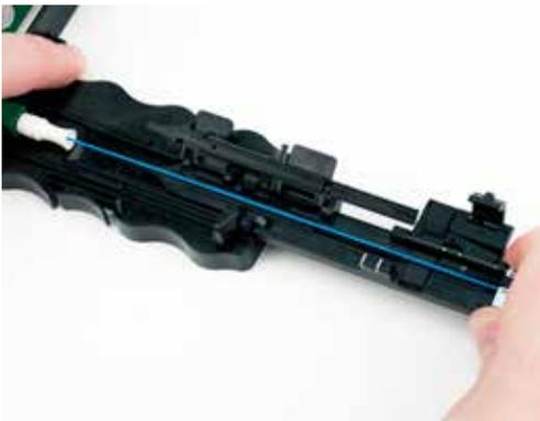
**Step 3 – Polish fiber tip with one turn of a handle, using the 3M Crimplok+ Nano Finishing Tool.**
