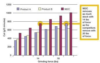
\*Projected due to standardisation of the data based on actual internal grinding force tests. 1 Lbs =  $0.45\,\text{Kgs}$
