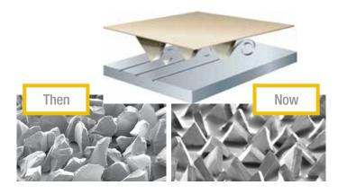
Triangular-shaped grain (right image) is electrostatically oriented to form sharp peaks, each acting like individual cutting tools that slice through metal, wear evenly and provide super-long life and consistency at any grinding pressure.
