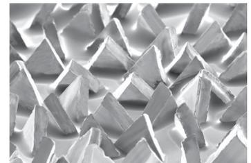
3M precision-shaped grain, engineered with ultra-sharp grain, cuts fast and lasts long. These triangular-shaped grains (right image) are electrostatically oriented to form sharp peaks, each acting like individual cutting tools that slice through metal, wear evenly and provide super-long life and consistency at any grinding pressure.
