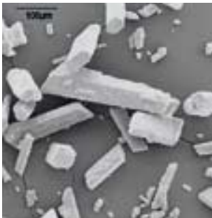
Conventional air-polishing powders • up to 200 µm particle size • should only be applied once, maximally twice, per year due to abrasivity
