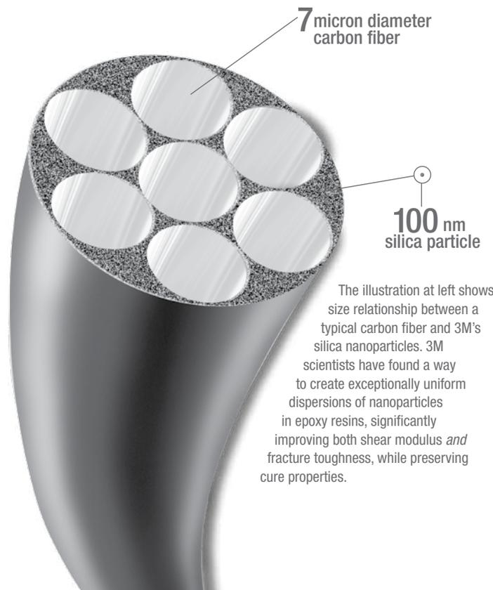
The illustration at left shows the size relationship between a typical carbon fiber and 3M's silica nanoparticles. 3M scientists have found a way to create exceptionally uniform dispersions of nanoparticles in epoxy resins, significantly improving both shear modulus *and* fracture toughness, while preserving cure properties.
