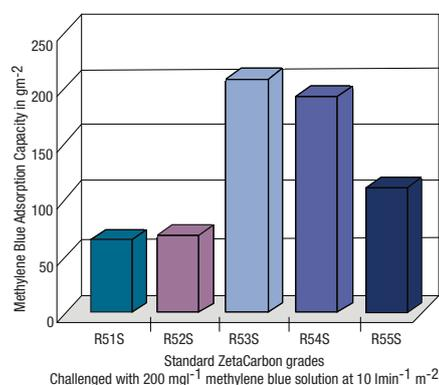
**Graph 2: Adsorption Capacity of 3M Purification ZetaCarbon R53S**
