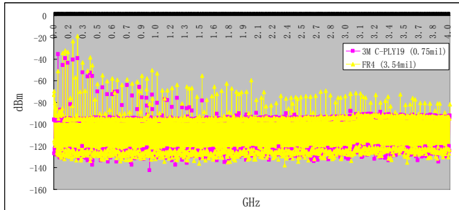
Fig. 10. comparison of the power noise frequency spectrum of the embedded capacitance and the conventional FR-4 material boards
