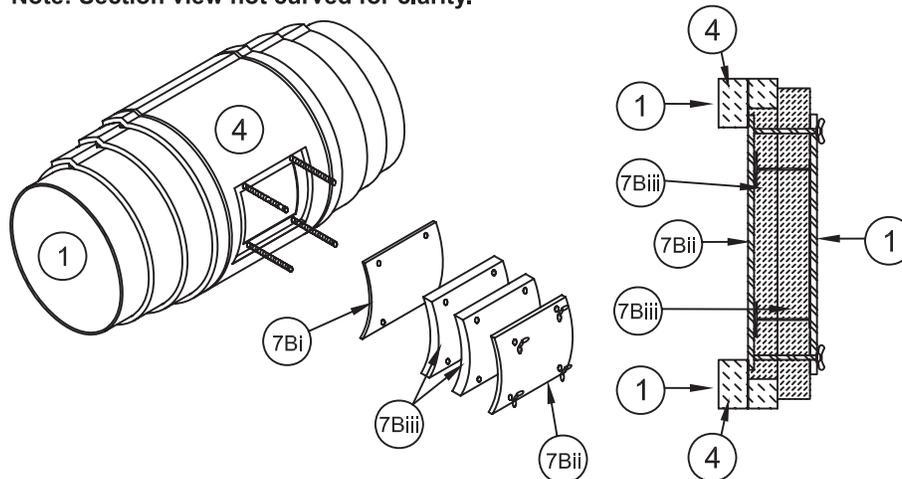
**Figure 4 – Field Fabricated Access Door Option B**
