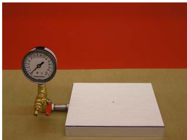
Pressure chamber with Kemlite FRP reefer roofing cover plate
