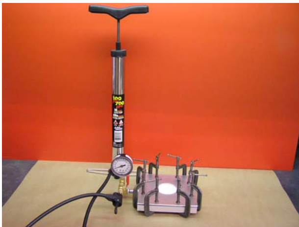
Tire pump used to pressurize chamber
