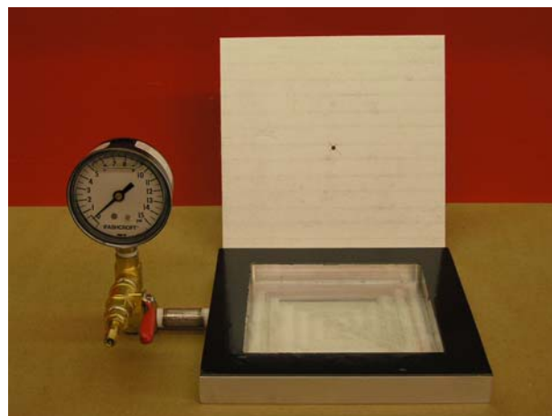
Pressure chamber with 3M™ VHB™ 5962 ready for cover plate
