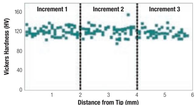
Fig. 4: Following the standard filling composite placement protocol, three consecutive 2 mm increments of Filtek™ Z250 Universal Restorative, A3, were cured for 10 seconds each. The specimen was hemisectioned and Vickers Hardness was determined with a micro indenter. The Elipar™ S10 LED Curing Light delivered consistently high hardness throughout the filling.
