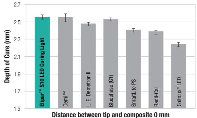
Fig. 7: The Elipar™ S10 LED Curing Light offers a high depth of cure compared to leading devices tested. Measured according to ISO 4049:2000.
