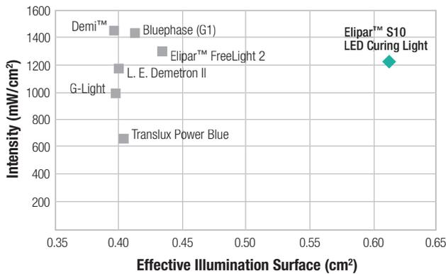
Fig. 5: Intensity is optical power divided by effective tip surface. The tremendous optical power of the Elipar™ S10 LED Curing Light allows keeping intensity very high, and offering a large effective surface at the same time.
