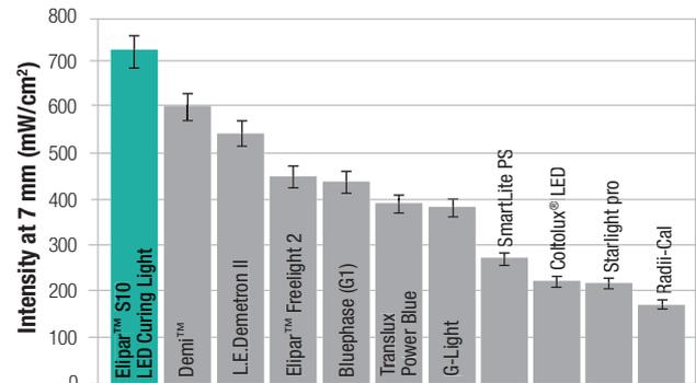
Fig. 2: The Elipar™ S10 LED Curing Light offers more intensity at the clinically relevant distance of 7 mm compared to leading devices tested. Measured with a spectrally resolving radiometer equipped with an integrating sphere (aperture 4 mm).
