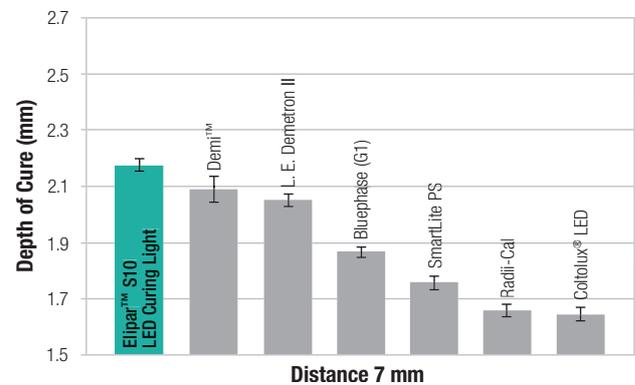
Fig. 3: Due to its more focused light output, the Elipar™ S10 LED Curing Light offers improved depth of cure when curing from a clinically relevant distance of 7 mm.
