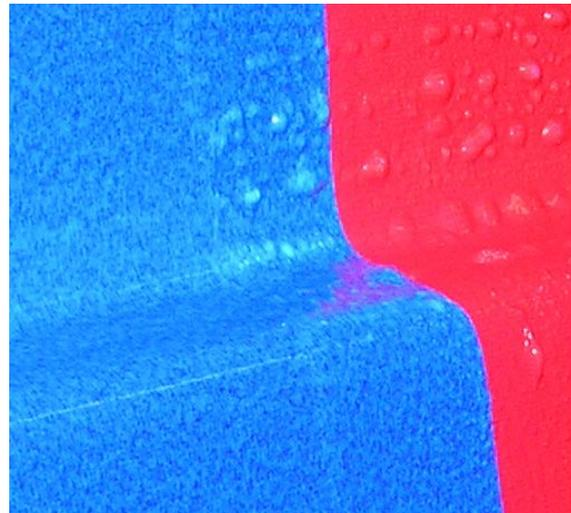
**⚠ CAUTION:** Re-heating of the film and re-rolling the film into the recess or corrugation is a quality control step to ensure the application is completed correctly and that all air bubbles are removed.
