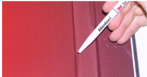
14. Multi panel graphics should be applied with an overlap between 3 and 7mm.
