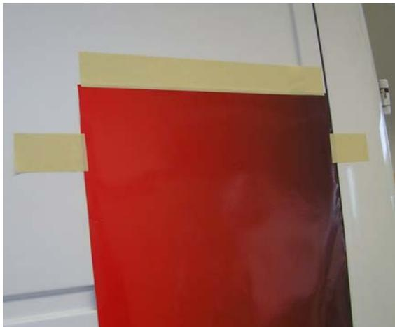
3. Remove the masking tapes from the sides. Roll the panel up to the top.
