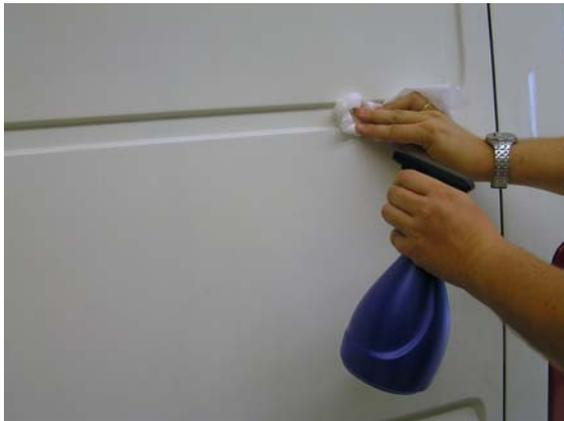
**Note:** Do not use alcohol based cleaning solvents e.g. isopropyl alcohol or methylated spirit as these can affect the adhesion of the film in the recessed area. Cleaning solvents, other than 3M™ Surface Preparation System, may also affect the expected adhesion and performance of the graphic film.
