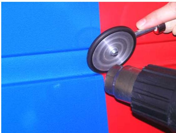
17. Re-heat the substrate again with the hot-air gun at a temperature of at least 80°C and press the film again with the small hand-roller.
