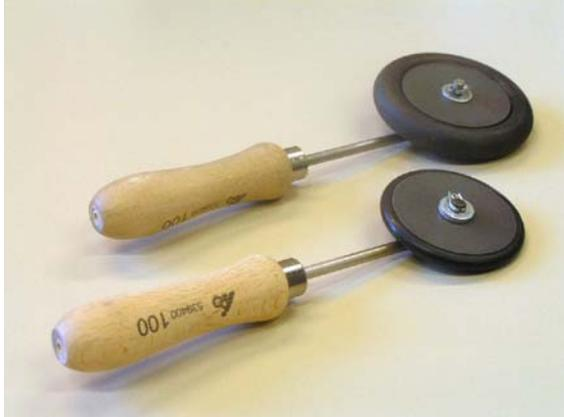
10. Use the big hand-roller for applying the film into the centre of the recess starting from the middle working towards the edges of the film.
