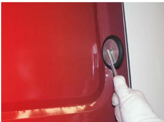
12. To complete the application, heat the film to a temperature of approximately 50°C and use the small hand-roller to close the remaining air channels between the film and the substrate.
