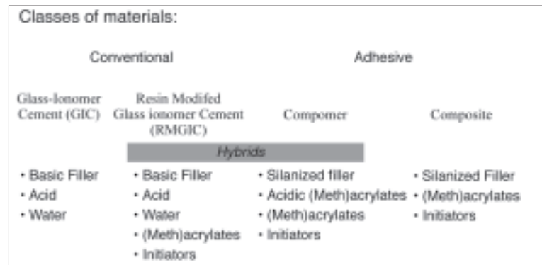
Figure 1. Glass ionomer-composite continuum; composition of material classes
