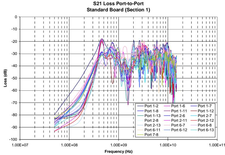
**Figure 5 – S21 of Typical Board (Courtesy of IBM)**
