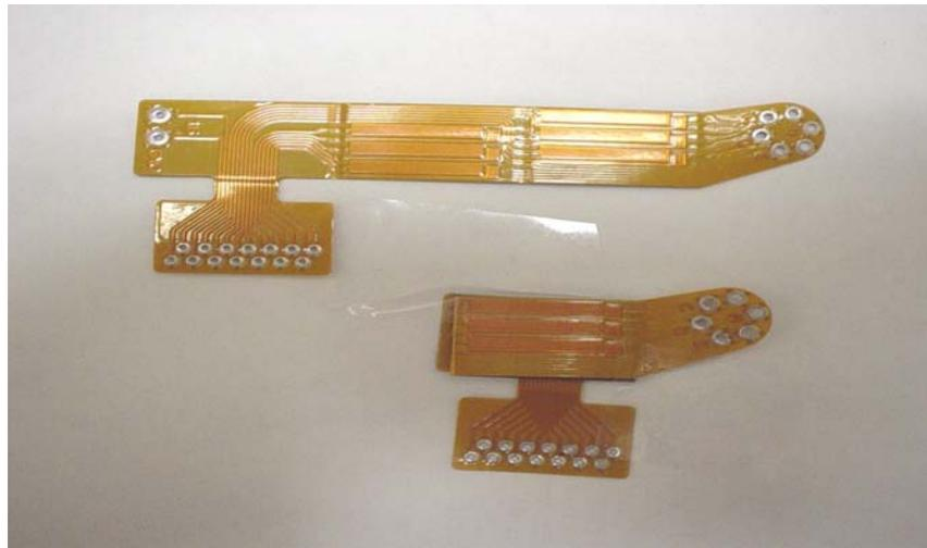
**Figure 13 – Embedded Capacitor Substrate Used as a Flex Circuit**
