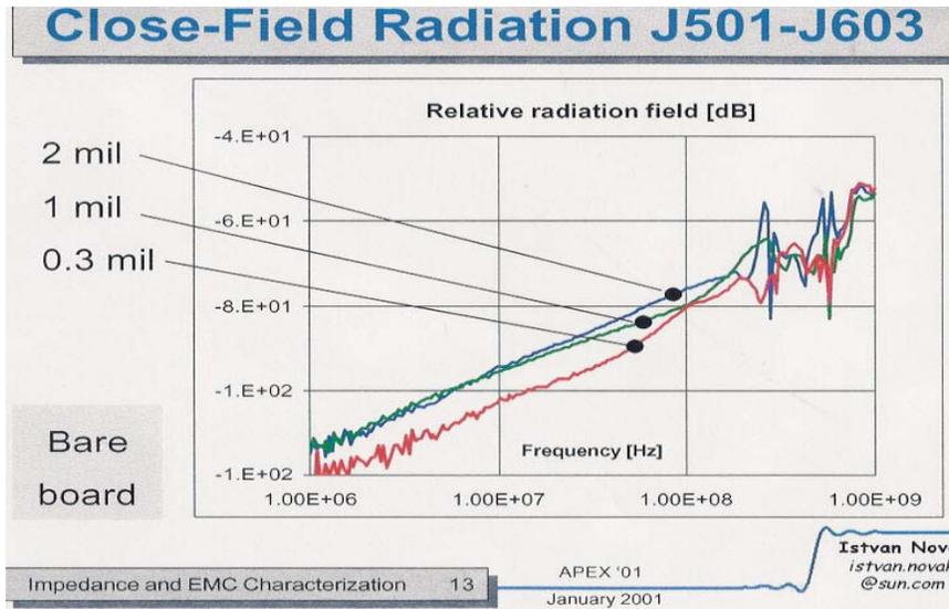
**Figure 3 – EMI vs. Frequency**
