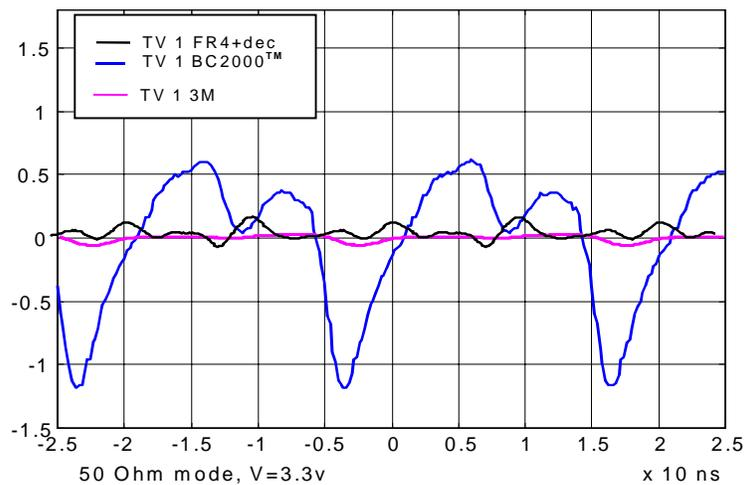
**Figure 9 – Power Plane Voltage Fluctuation**
