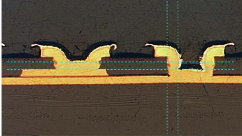
**Figure 10 – Microvias in Test Board
