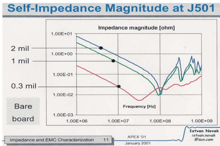
Figure 1 – Self-Impedance vs. Frequency
