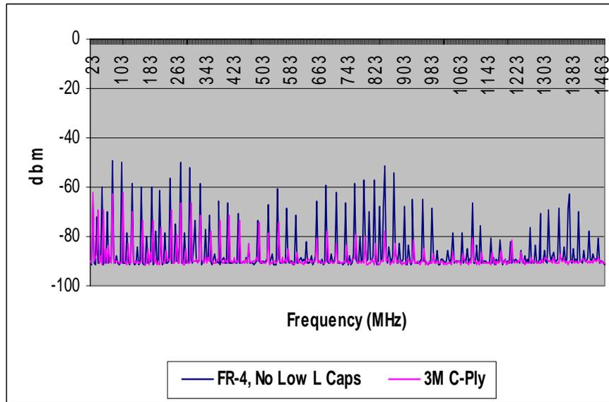
**Figure 7 – Power Bus Noise vs. Frequency**
