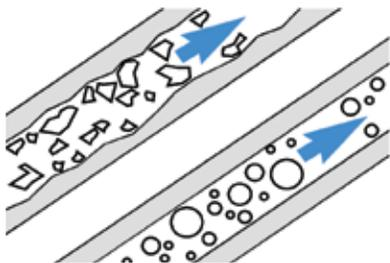
Unlike irregularly-shaped fillers, 3M glass microspheres roll easily over one another. This helps increase volume loading capacity, reduce shrinkage, reduce warpage and lower resin demand. It can also help reduce warpage in many molded plastic parts.
