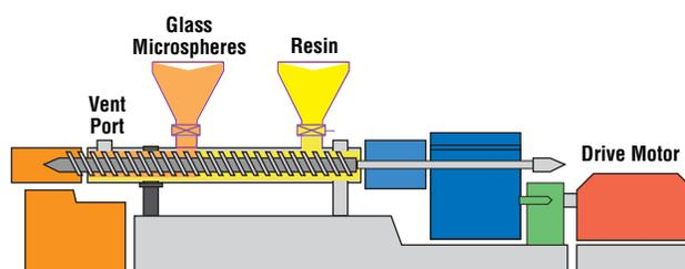
Fig. 1 Typical setup on a twin-screw extruder
