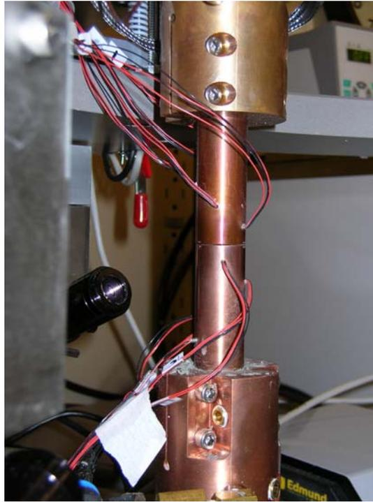
FIGURE IV. PHOTOGRAPH OF THE UNWRAPPED METER BARS
