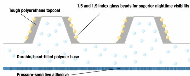
*This cross-section of 3M™ Stamark™ Tape Series 270 shows how 3M's advanced technologies make this tape a durable value for intersection safety.*
