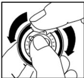
Using your fingertip, apply a small amount of talcum powder to the inside surface of the flexible edge of the diaphragm. This will facilitate assembly and maintain smooth and quiet low/high frequency alternation.
