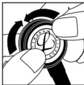
Slowly roll the rim around and over the chestpiece edge using both thumbs, moving in opposite directions around the chestpiece.
