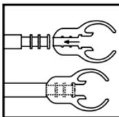
eartube. The eartips are pushed on to the end of the eartube and snapped firmly into place. To remove, pull firmly on the eartip.
