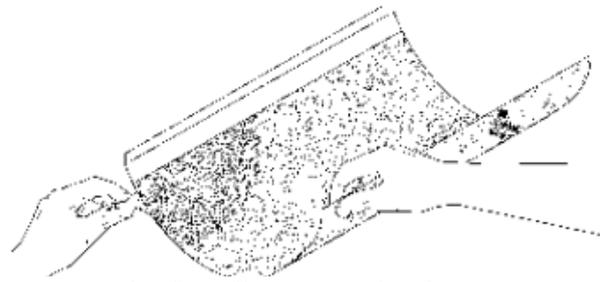
Figure 6. Lift the Graphic and Peel Back the Liner
