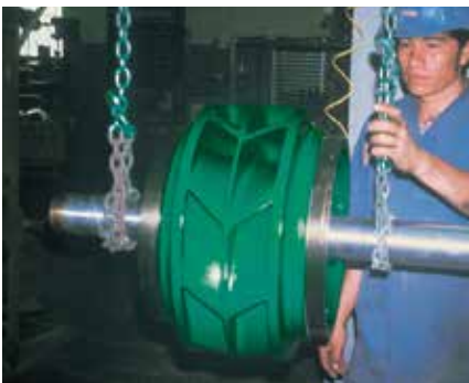
Application of 3M™ Scotchkote™ FBE Coating 134 custom coating on a turbine.
