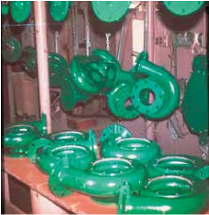
Pump volutes protected against corrosion with 3M™ Scotchkote™ FBE Coating 134.
