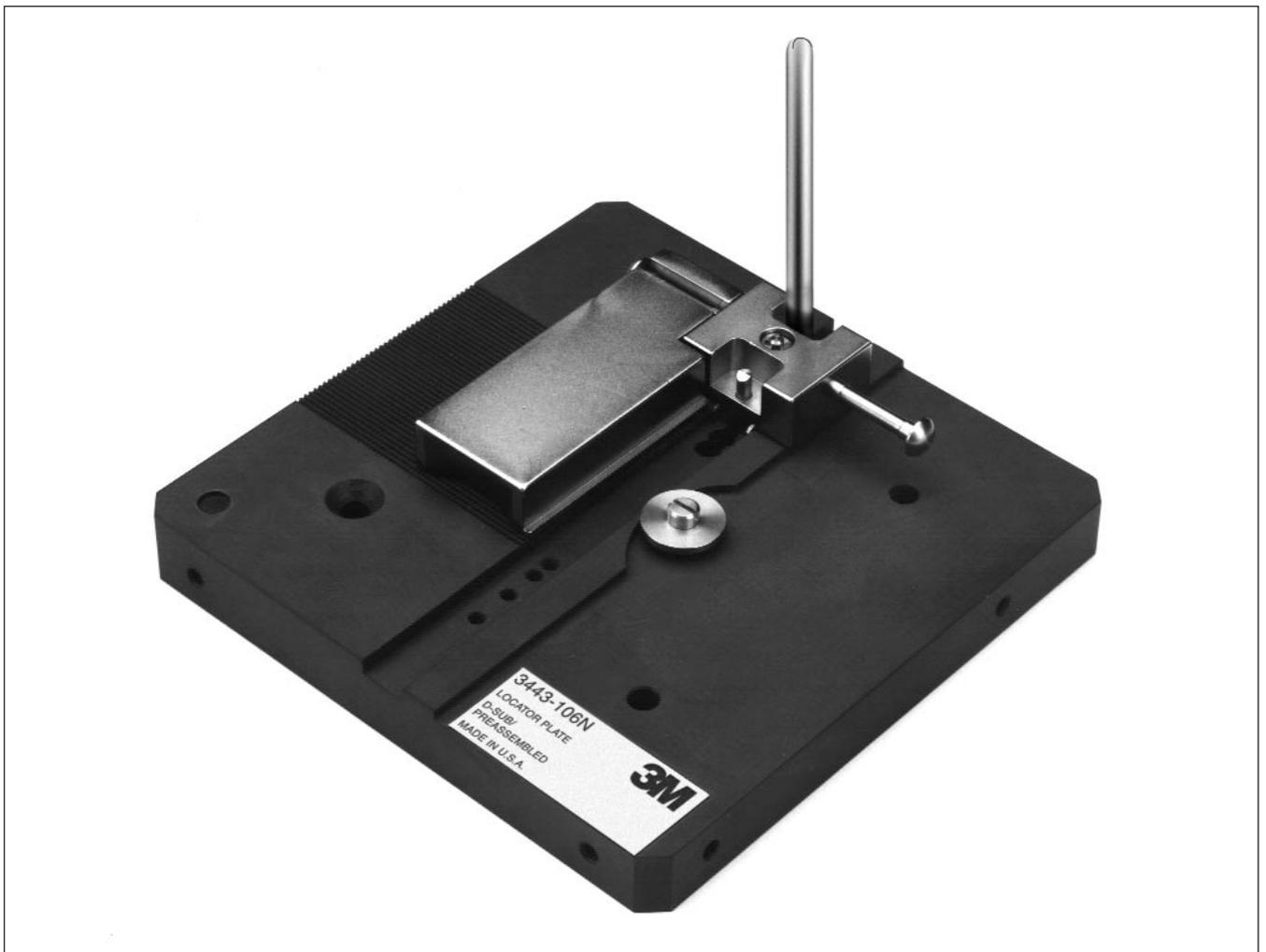
The 3M Locator Plate 3443-106N is designed to aid in the assembly of the preassembled and two-piece 3M™ Delta Connector and pin 9 through 37 position connectors. End-to-end, as well as daisy chain assemblies, can be made. Set-up and assembly instructions are based on termination procedures with the 3M manual and pneumatic presses.
