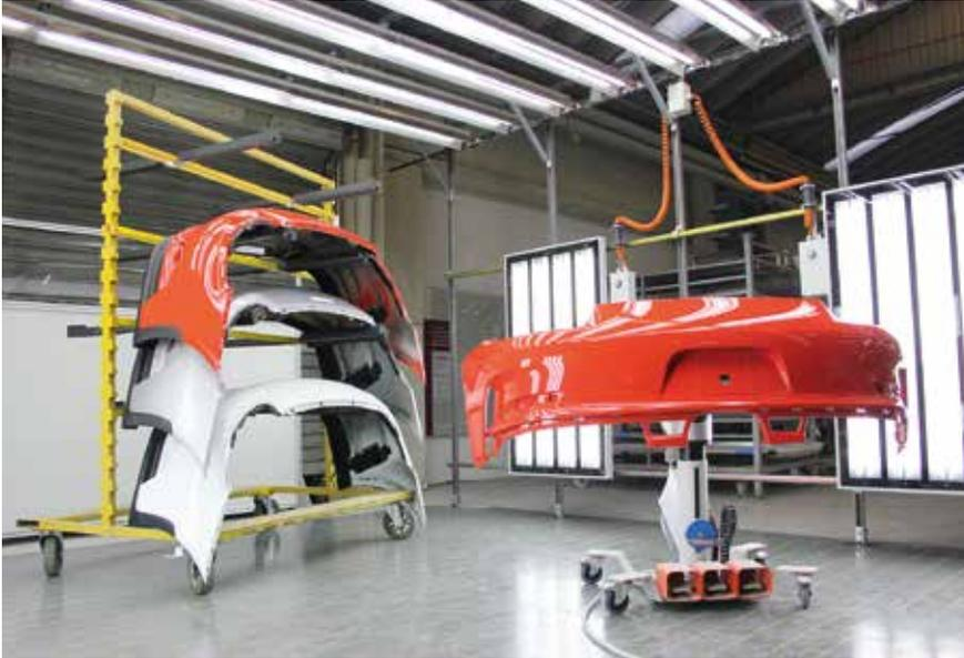
**Fig. 2.** View of rear apron production in Hörsching, Austria. The components are not only produced here but also receive a class A paint finish. The site specializes in short-run production of automotive exterior parts (© Polytec Group)
