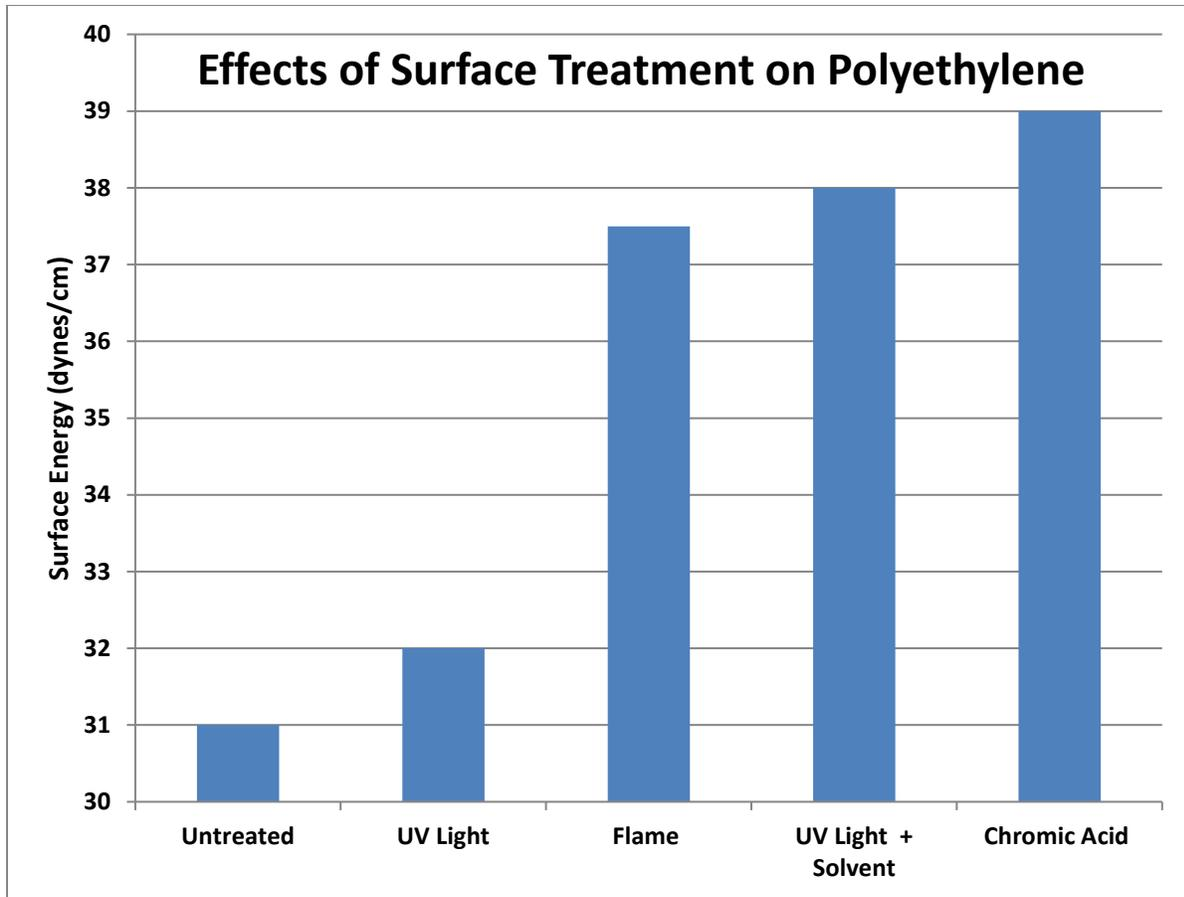
*Increase in surface energy of Polyethylene after several common surface treatment methods.*
