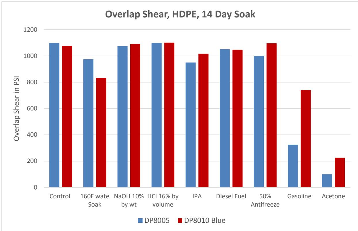
***Bonding Strength of 3M™ Scotch-Weld™ Structural Plastic Adhesive DP8005 and 3M™ Scotch-Weld™ Structural Plastic Adhesive DP8010 Blue on HDPE after various environmental challenge conditions.***
