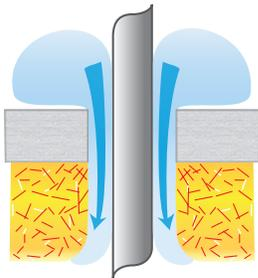
A draft fan  $\Delta P$  of 0.35" of water draws outside air through a nominal 1 ft<sup>2</sup> gap at a rate of 1.92 lbs/sec., every day, every month, every year. Tube seals made using Nextel ceramic textiles help stop the ingress of air.
