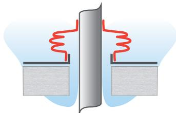
Tube seals are designed to flex to allow for the expansion of the process tube relative to the furnace roof. Tube seals made using Nextel ceramic textiles remain flexible for years of continuous operation up to 2200°F.
