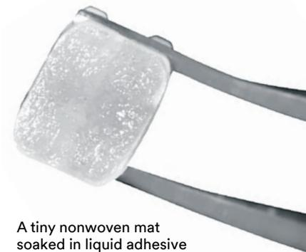
A tiny nonwoven mat soaked in liquid adhesive resin is the secret behind the flash-free performance of 3M's APC™ Flash-Free Adhesive coated brackets.
