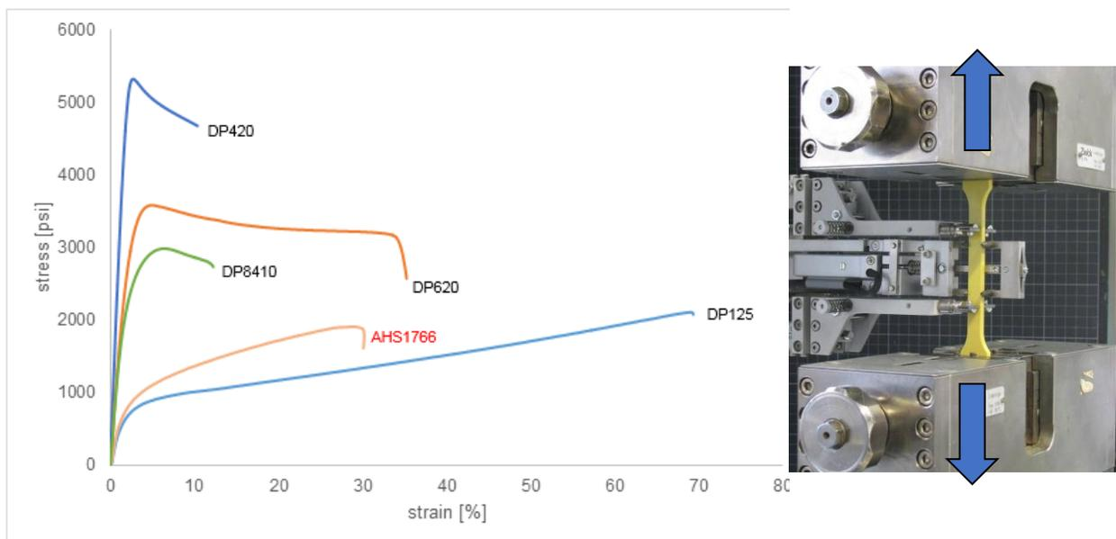
Figure 8: The image above is showing some stress-strain curves of a selection of adhesives. For this, load is applied to a dumbbell-shaped specimen as shown on the right side. The curves represent the different families of adhesives. Toughened epoxy (DP420), toughened polyurethane (DP620), methacrylate (DP8410), flexible Urethane (DP6330NS) and flexible epoxy (DP125)
